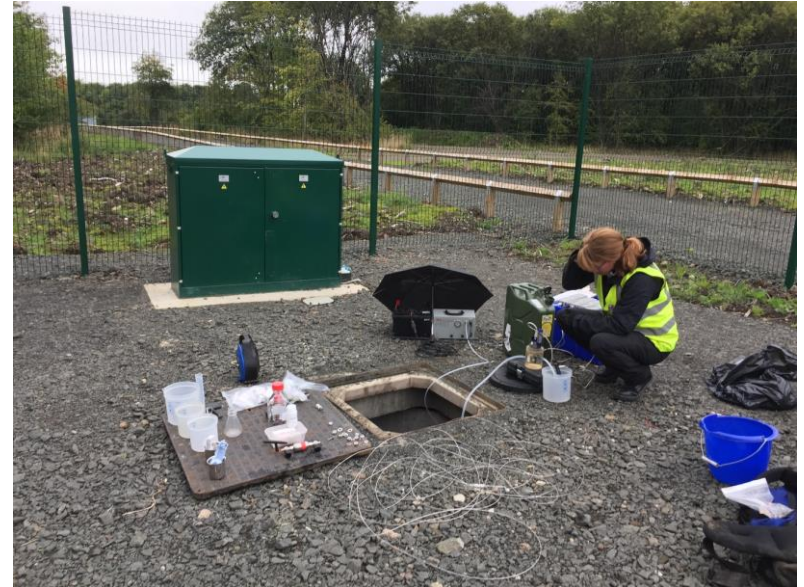
Groundwater sampling of a mine water borehole at the UK Geoenergy Observatory in Glasgow, BGS©UKRI
