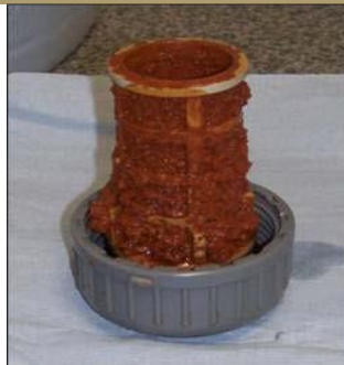
David Banks/TCA. Effect of oxygenation of mine water on a heat exchanger
