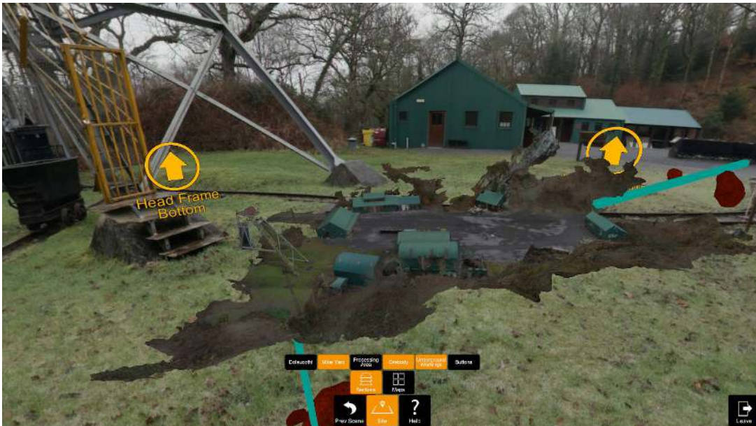
Fig. 2: 3D model of mine yard and underground workings orientation & navigation tool
